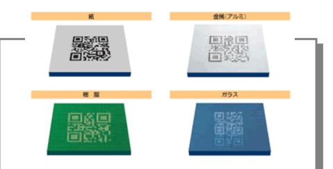
Besides symbols that are printed on papers, dot-pattern 2D symbols marked on metal, resin or glass materials are also supported.
